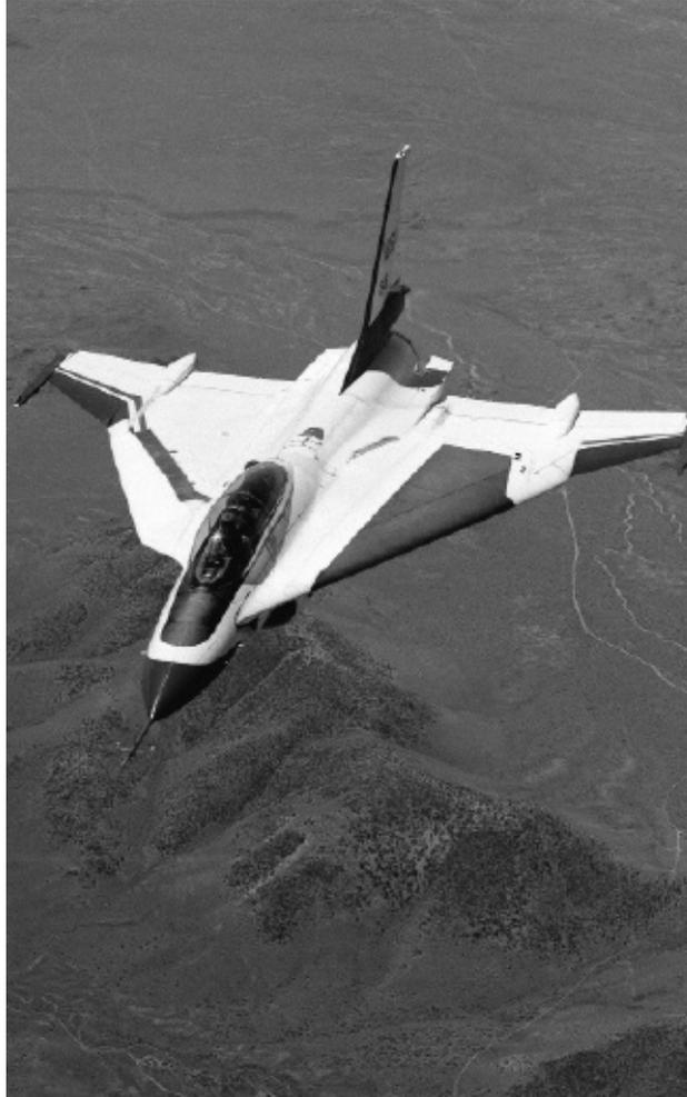
**Case-12 Cover Image:** *The F-16XL-2 was one of two test aircraft that NASA Dryden used in the 1990s to test the application of laminar flow at supersonic speeds. NASA.*
