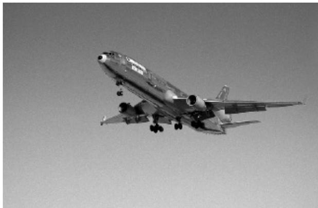
*A computer system known as Propulsion Controlled Aircraft is tested aboard an MD-11 airliner in 1995 at the Dryden Flight Research Center. NASA.*
