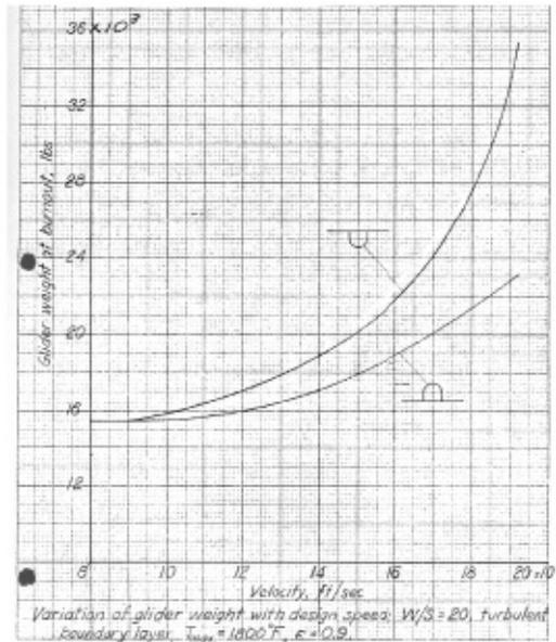
*This 1957 Langley trade-study shows weight advantage of flat-bottom reentry vehicles at higher Mach numbers. This led to abandonment of high-wing designs in favor of flat-bottom ones such as the X-20 Dyna-Soar and the Space Shuttle. NASA.*
