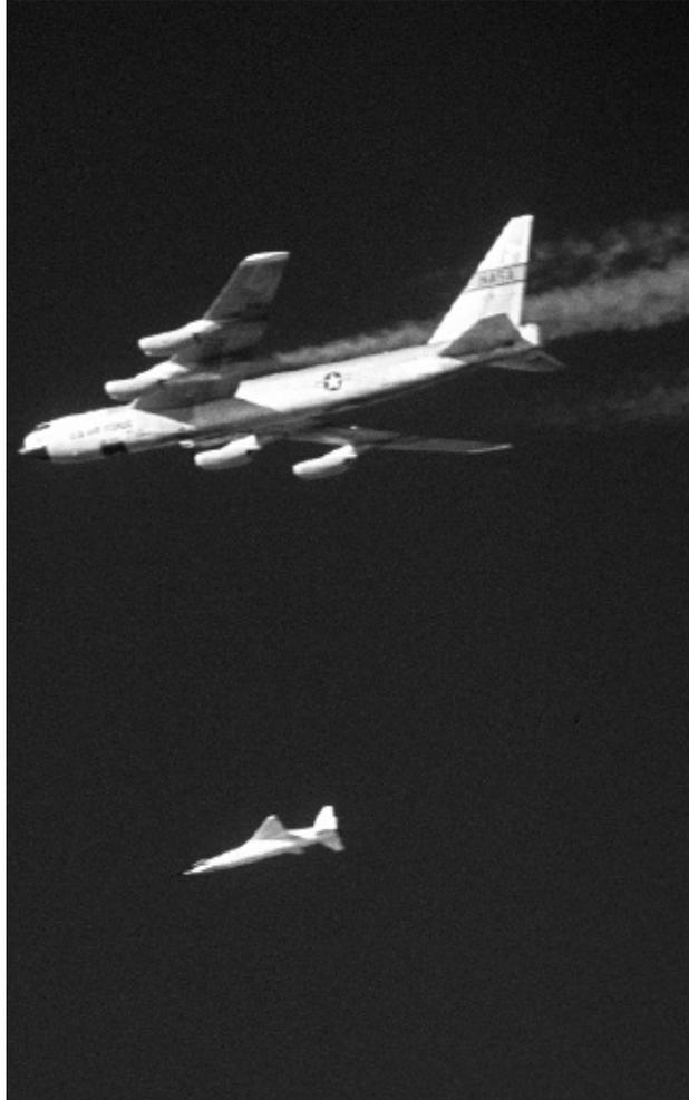
**Case-9 Cover Image:** *The X-43A Hyper-X test vehicle drops away from its Boeing NB-52B mother ship in November 2004, beginning its flight to Mach 9.7. NASA.*
