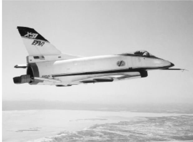
*The X-31 aircraft, showing thrust vectoring paddles. NASA.*
