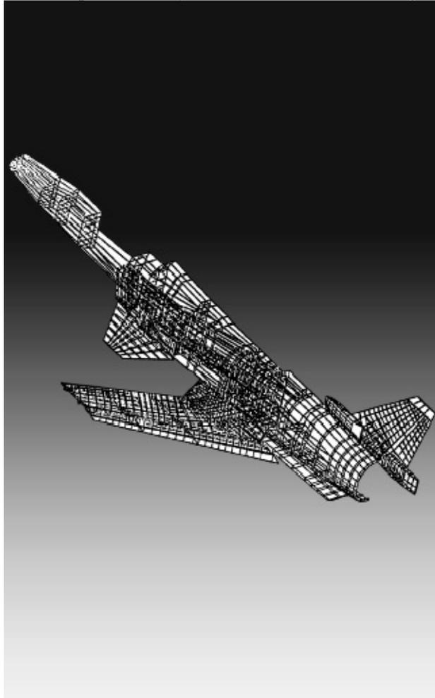
**Case-8 Cover Image:** NASTRAN model of the X29A aircraft. NASA.
