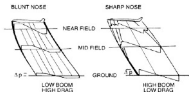
Figure 6. Low-boom/high-drag paradox. NASA.
