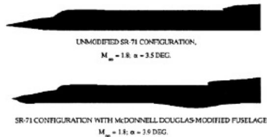
Figure 8. Proposed SR-71 low-boom modification. NASA.
