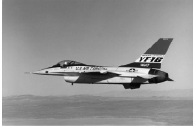
*The General Dynamics YF-16 prototype Lightweight Fighter (LWF) in flight over the Edwards range. USAF.*
