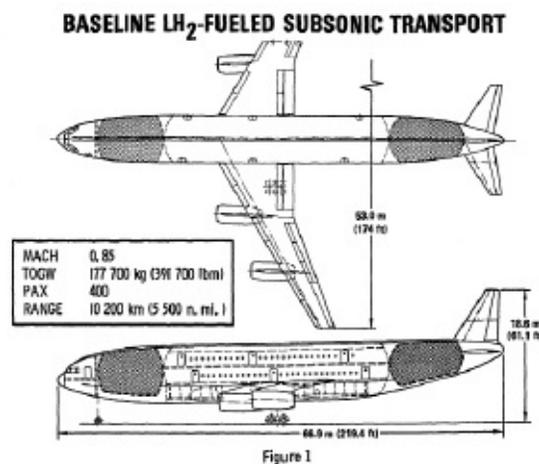
*A 1978 NASA conceptual design study for a liquid-hydrogen-powered jetliner. Note the large volume required by liquid hydrogen, compared with conventional hydrocarbon-fueled airliners. NASA.*
