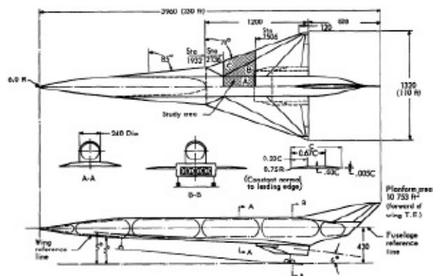
*A hypersonic scramjet configuration developed by Langley experts in the 1970s. The sharply swept double-delta layout set the stage for the National Aero-Space Plane program. NASA.*
