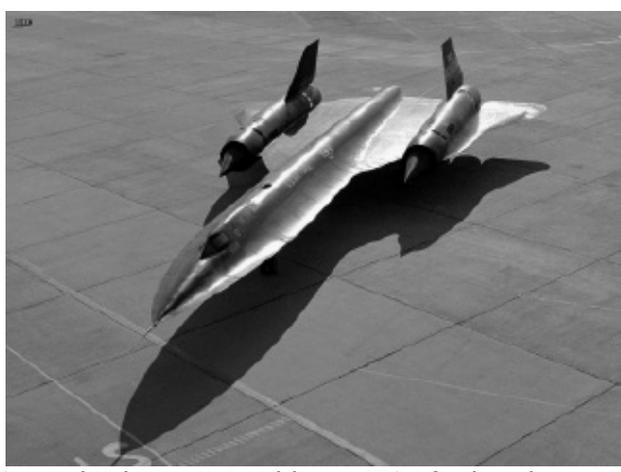
*The YF-12C used twin Pratt & Whitney J58 afterburning engines. NASA.*
