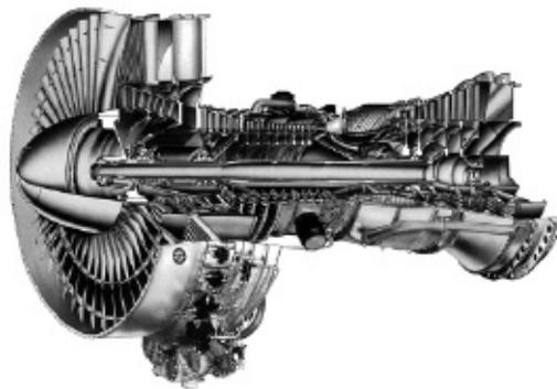
*The classic Pratt & Whitney JT9D engine interior and its major components: the fan, compressor, combustion chamber, turbine, and nozzle. Pratt & Whitney.*
