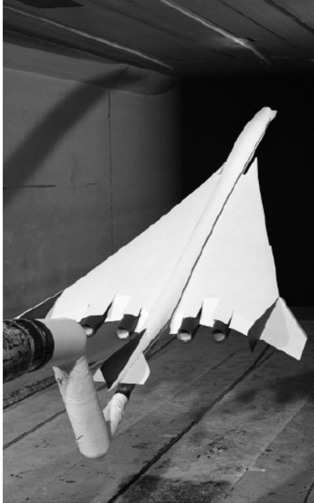
**Case-4 Cover Image:** Aerodynamic model of NASA's SCAT-15F supersonic transport design attached for a subsonic wind tunnel test in 1969. NASA.
