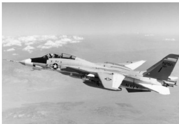
*The Grumman F-14A Tomcat naval fighter marked the maturation of the variable wing-sweep concept. This one was assigned to Dryden for high angle of attack and departure flight-testing. NASA.*
