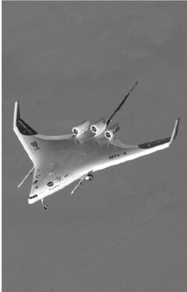
**Case-1 Cover Image:** *The X-48B subscale demonstrator for the Blended Wing-Body (BWB). The BWB may represent the next extension of the swept and delta wing, to transform flight away from the rule of the “tube and wing” jetliner. NASA.*
