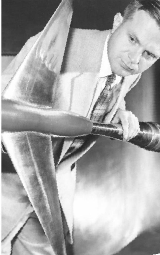
**Case-2 Cover Image:** *Whitcomb evaluates the shape of one of his area rule models in the 8-foot High Speed Tunnel. NASA.*
