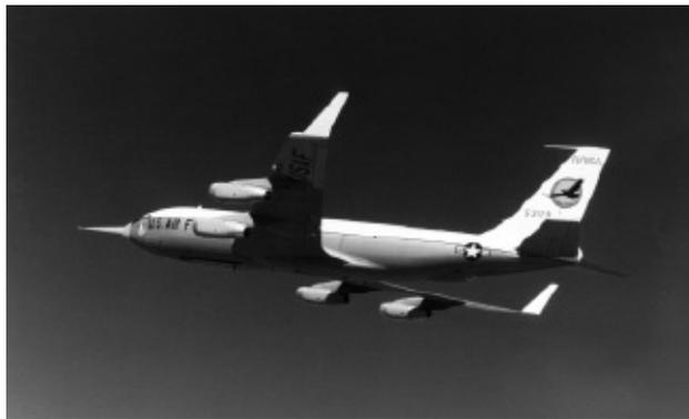
*The KC-135 winglet test vehicle in flight over Dryden. NASA.*
