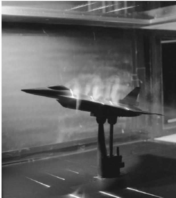
*An F-16XL flow visualization test. This F-16 Scamp model was tested in the NASA Langley Research Center Basic Aerodynamics Research Tunnel. This was a basic flow visualization test using a laser light sheet to illuminate the smoke.*
