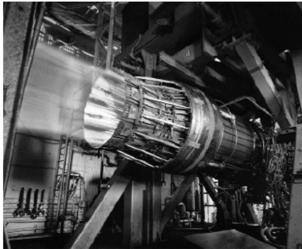
*The Digital Electronic Engine Control system was tested on a Pratt & Whitney F100 turbojet, similar to the one shown here undergoing a hot fire on a test stand. Pratt & Whitney.*
