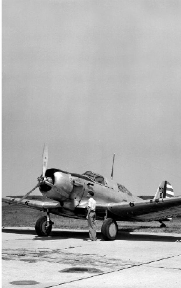
**Case-11 Cover Image:** An NACA cowling on a Northrop A-17A at the Agency's Langley Laboratory in 1939. The NACA cowling was its signal contribution to integrating propulsive and aerodynamic design. NASA.
