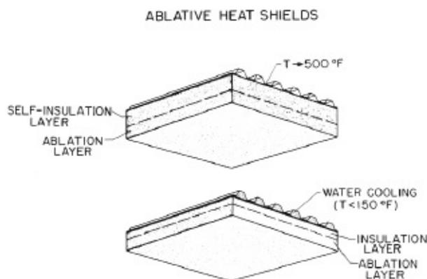
NASA concepts for passive and actively cooled ablative heat shields, 1960. NASA.
