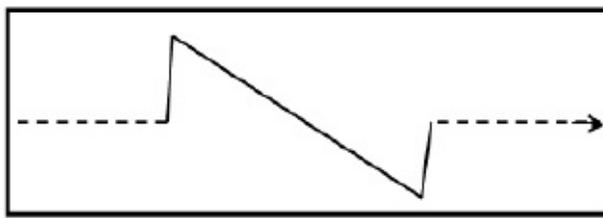
Figure 1. Simplified N-shaped sonic boom signature. NASA.
