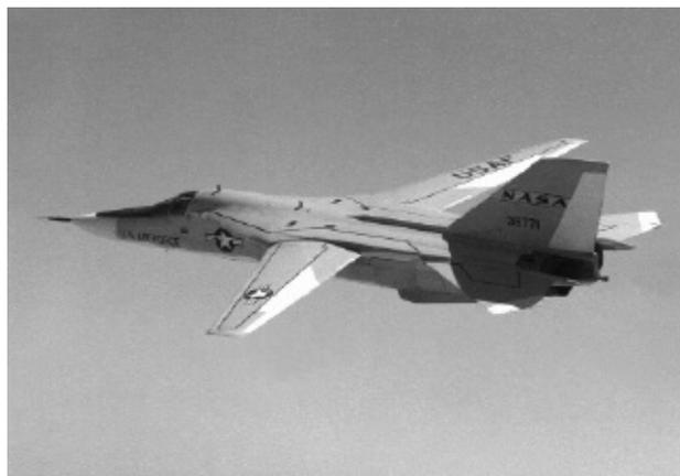
*The General Dynamics F-111A was the first production aircraft to use a self-adaptive flight control system. NASA.*
