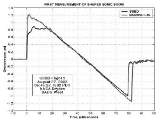
Figure 9. Normal and flattened F-5E sonic boom signatures. NASA.
