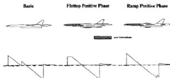
Figure 7. Proposed modifications to BQM-34 Firebee II. NASA.
