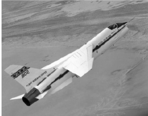
*For the DFBW F-8 program, the Flight Research Center removed all mechanical linkages and cables to the flight control surfaces. NASA.*
