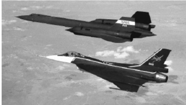
*In 1995, the Dryden Flight Research Center used an F-16XL to make detailed in-flight supersonic shock wave measurements as near as 80 feet from an SR-71. NASA.*
