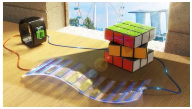
Shadow-effect energy generators, like the one illustrated here, could someday be used to produce power from the difference between bright spots and shady areas. The greater the contrast between light and dark, the more energy such generators provide.
