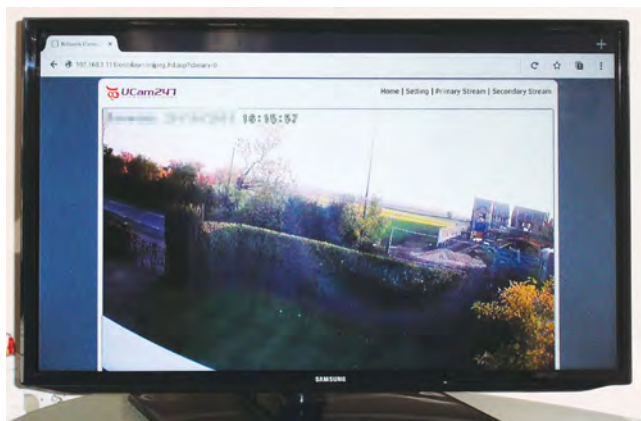
Fig.4. The IP camera video feed and setup screens could then be accessed using its IP address in the browser
