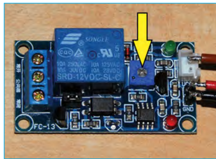
Fig.6. Use this pot to set the switching level
