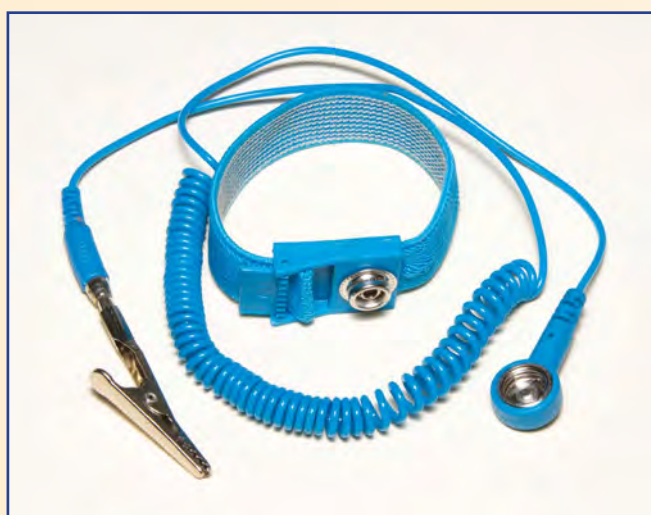
Fig.3. This anti-static wristband has a crocodile clip lead rather than a mains earth plug. It is primarily intended for use when building and servicing PCs, but it is usable when building electronic projects
