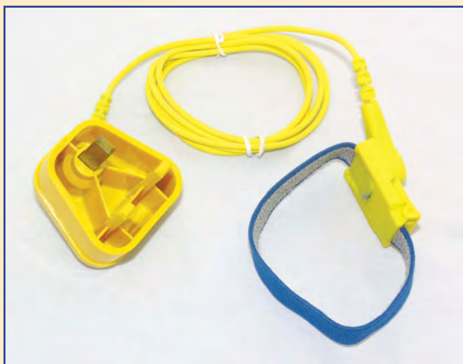
Fig.2. An anti-static wristband, complete with its lead and mains earth plug. For safety reasons there is a resistance of several megohms between the wristband and the plug
