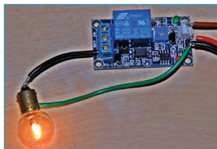
Fig.8. (top) Module turns light on for input above pre-set level (bottom) or on for input below a pre-set level – note the green LED
