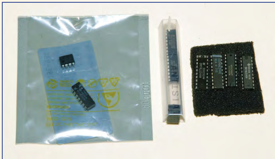
Fig. 1. Three types of anti-static packaging. The bag and the tube insulate the devices within from static charges, whereas the conductive foam effectively short-circuits all the pins together so that no significant voltage can exist between them
