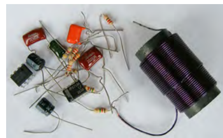
Fig.5. Contrast between passive inductor used in loudspeakers and parts to make an active filter crossover
