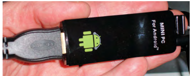
Fig.1. This £20 Android Mini PC dongle turns an HDMI TV into a fully-fledged Android computer with Wi-Fi, Bluetooth and USB
