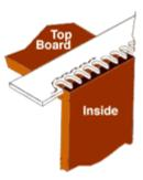
You can then join the boards together at the joints securing with glue and clamping overnight.
