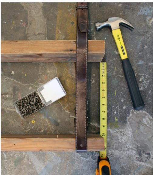
6. Hold the second board in place so the backside is also exactly 10" apart from the first boards (this ensures the boards are level) and hammer the nails into the center of the belt where it hits the backside of each board. Repeat on the other side.
