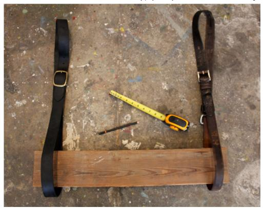
3. When you have the belts in the right place, hold the first belt so it can't move and turn the plank over so the underside is facing up. Hammer three nails into the belt, making sure the belt stays aligned with the 2" line. Repeat with the other belt on the left side.
