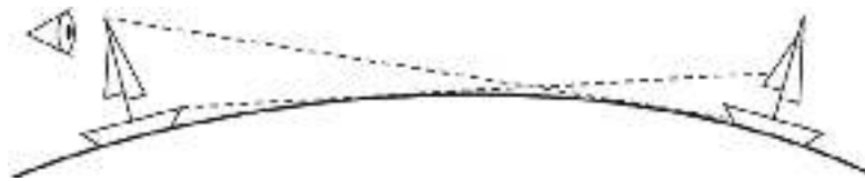
Line of sight from ship's deck and from the top of a ships mast.
